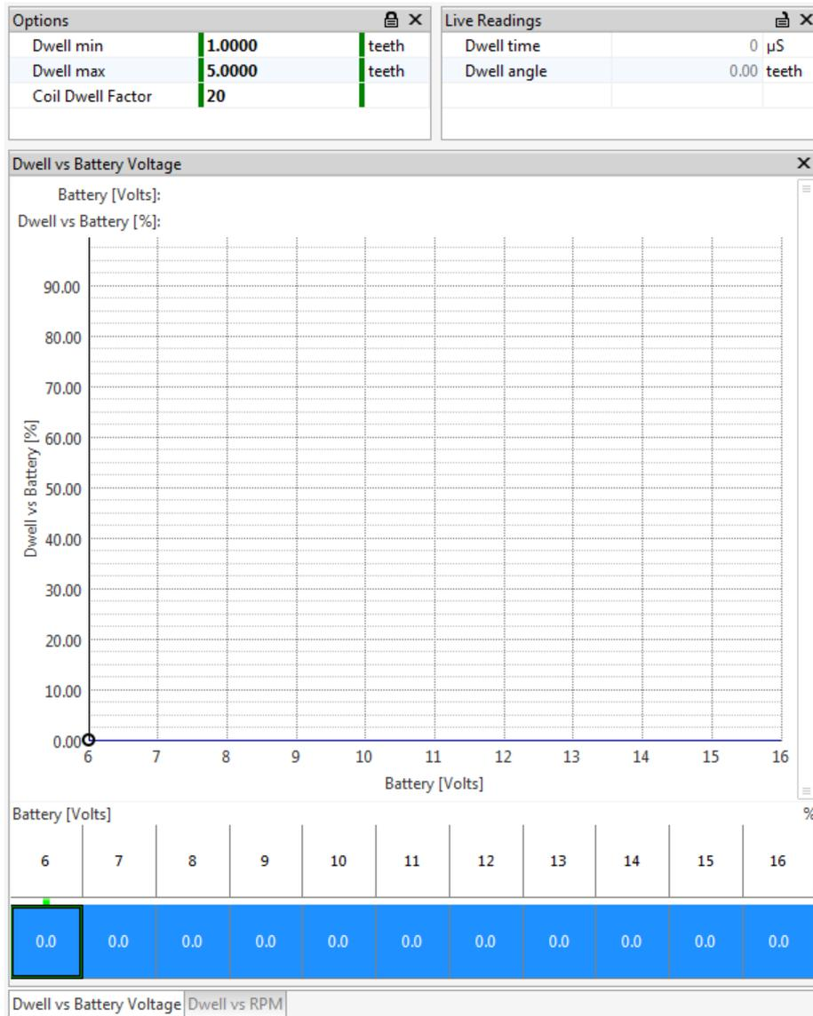
The coil dwell time is set by option **Coil Dwell Factor**. This is a unitless value typically 20 - 25 for a DIS coil pack. Charge times can be varied with respect to battery voltage and engine speed using the **Dwell vs Battery table** and **Dwell vs Speed table**. Setting these table values to 100% gives a constant dwell time.
