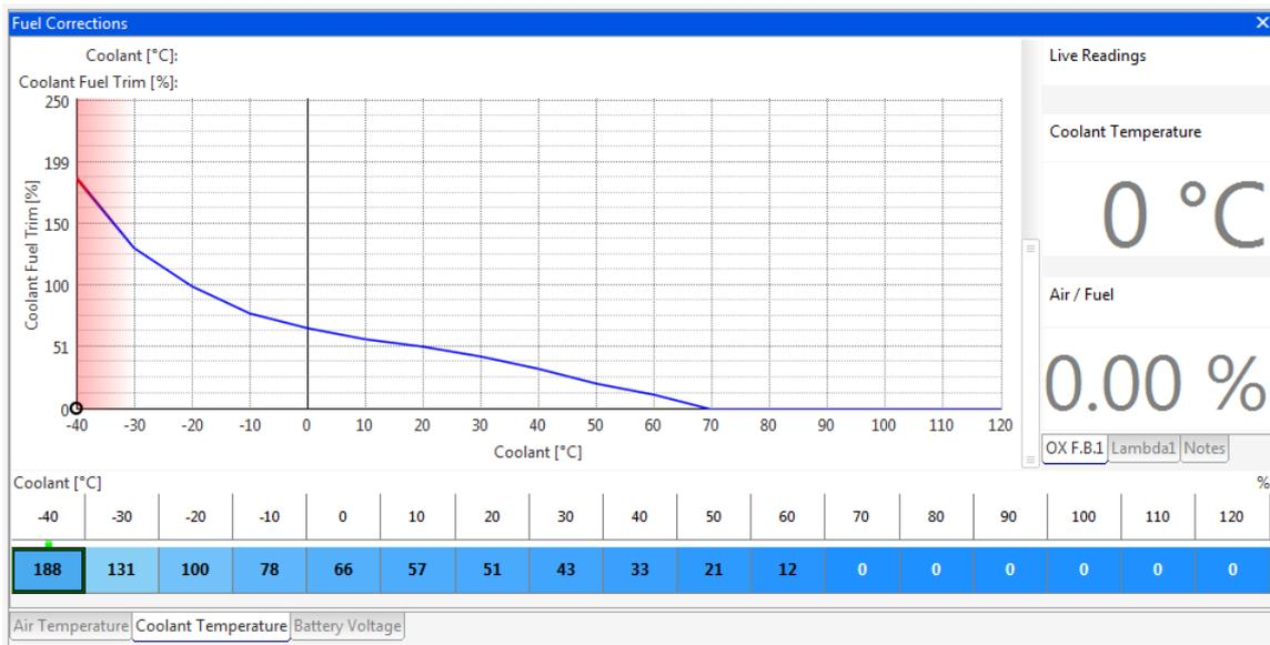
When the engine is cold, it requires an extra amount of fuel. This extra fuel is added as a percentage set in the **Coolant Fuel Trim table** of percentage increase against engine coolant temperature.
