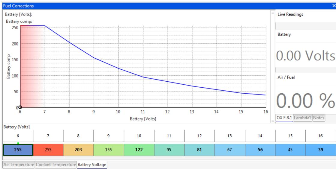
The battery voltage compensation data can usually be supplied by the injector manufacturers. For example, the Weber IW 058 injector data is for 3bar fuel pressure,
