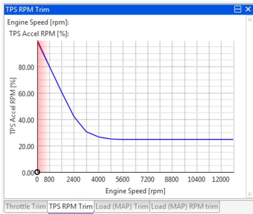
Engines usually require less acceleration fuel at high rpm, so the **TPS Accel RPM table** and **Load Accel RPM table** describe the percentage of the calculated fuel supplied at differing engine speeds.
