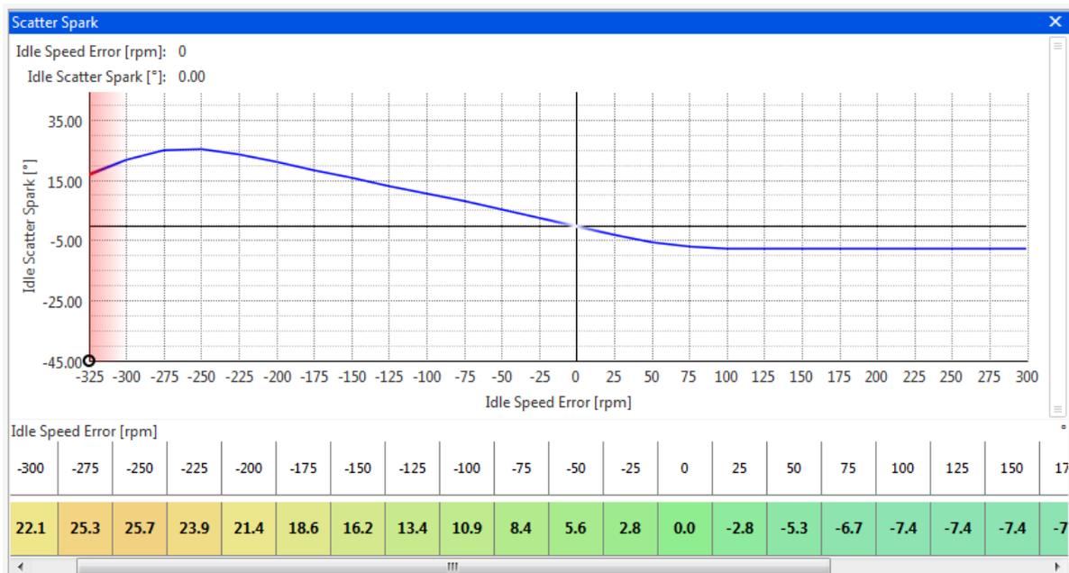
The **Idle Scatter Spark Table** shows the change in ignition timing based upon rpm away from the target engine speed. When the engine speed is higher than target negative values are required to
