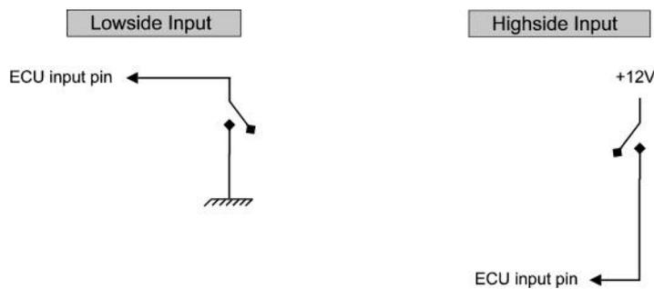
If an input is to be switched at the same time as something physical eg a solenoid for ALS, then the physical input switch can both turn on the solenoid and give an input to the ECU.
