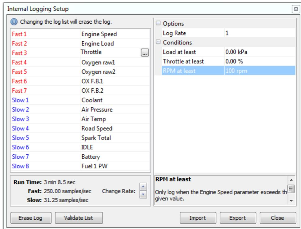
Logging can be triggered to start and stop dependent on engine conditions;
