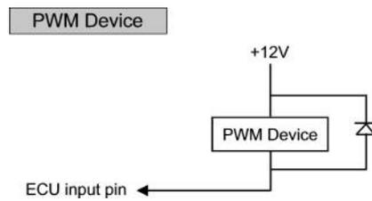
There are two types of input for the ECU, highside and lowside. Most inputs are highside. Contact Omex for advice.
