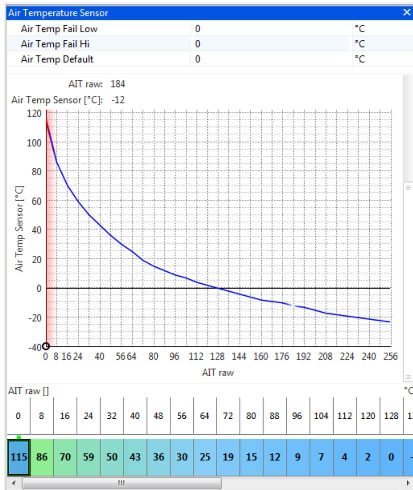
The air temperature sensor used by the Omex ECU is a resistive sensor. The raw output of this sensor is calibrated in the ECU to give the information in a more usable form, °C. Sensors are calibrated in the **Air Temp Sensor table**. The values for many sensors are known but you may need to calibrate your sensors. It is essential that these sensors are calibrated correctly as many functions are temperature based.
