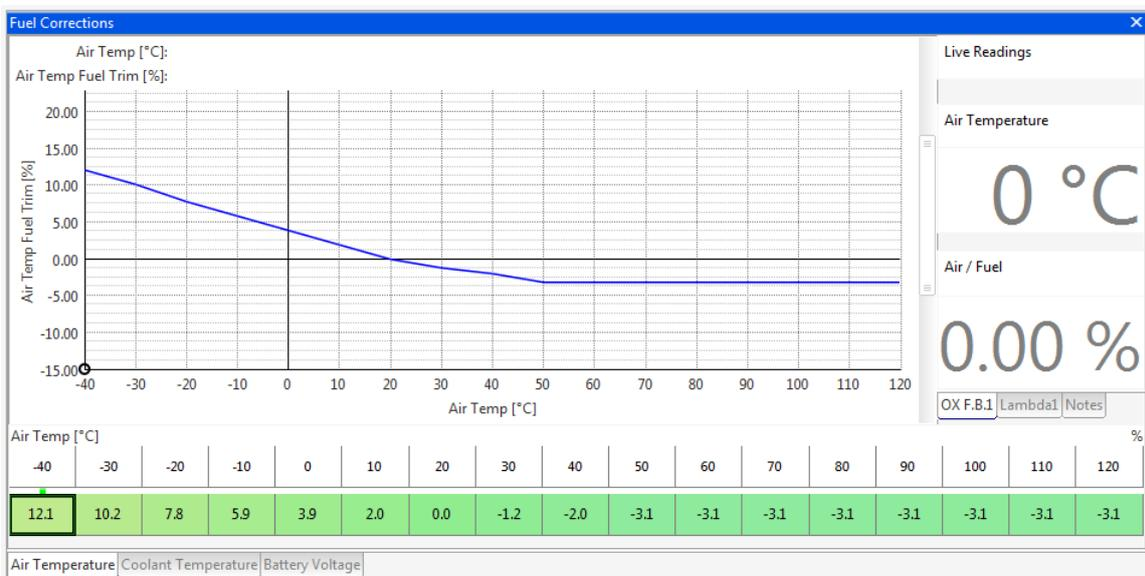
If you wish to change the fuelling with air inlet temperature, then the **Air Temp Fuel Trim table** allows the user to make a percentage change in fuel based on AIT.
