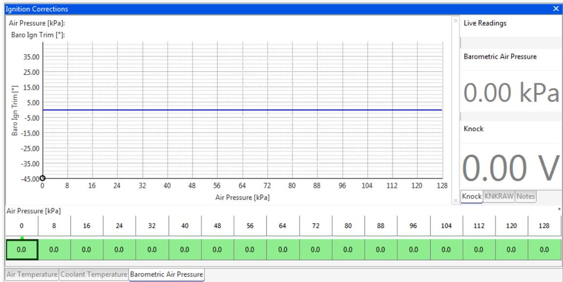
The fuel and ignition can be trimmed to allow for changes in barometric pressure as sensed by a 1bar pressure sensor. The ignition trim is defined in the **Baro Ign Trim table**. The fuel trim values are a known mathematical equation so are inbuilt and are non-adjustable.
