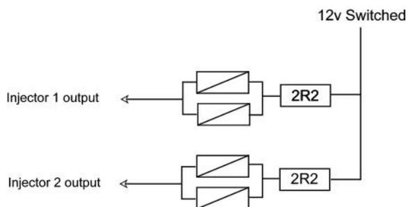
PWM devices driven from the FUEL1-8 outputs require a diode between their output and power.
