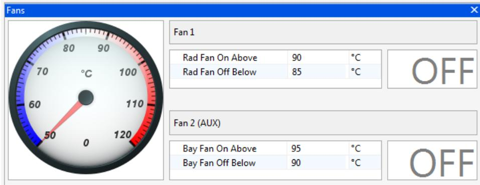
The ECU has two software outputs switchable on coolant temperature values. These would normally be used for cooling fans. The two outputs may be set to two different fans or set at different temperatures for twin speed fans.
